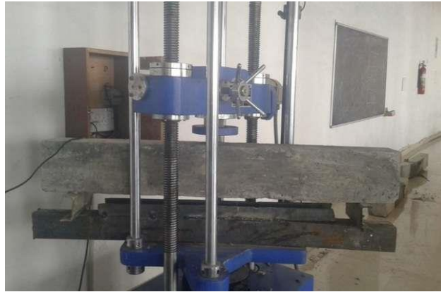
Figure 3.8 Experimental Setup for Testing Beams
