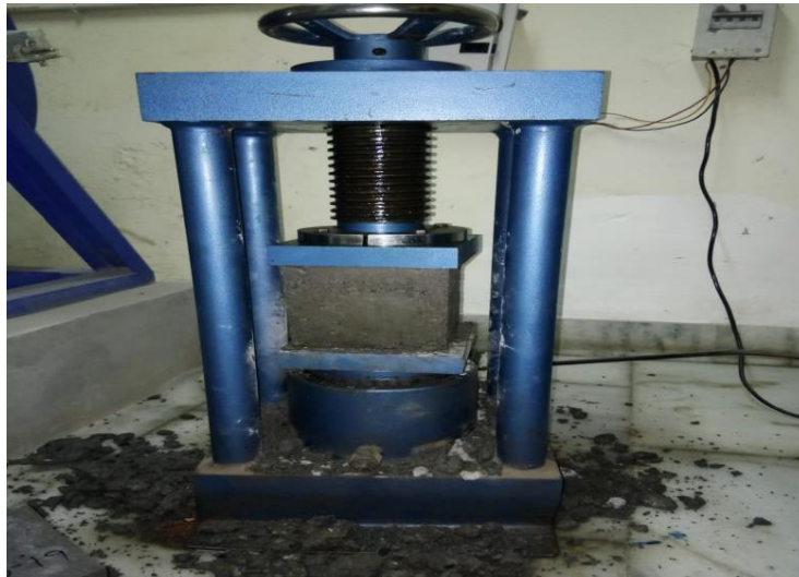
Figure 3.4 Cube during compressive strength test
