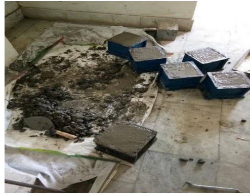
Figure 3.2 Casting of cubes
