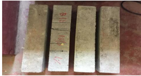
Fig 4.3: Prisms after flexural testing
