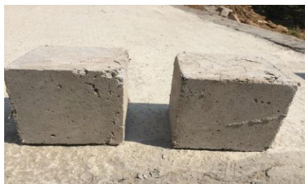
Fig 4.2: Cubes after compressive test
