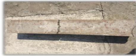
Fig 5.3: Failure of prisms after testing
