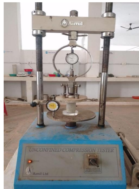
Figure 8: UCC testing machine
