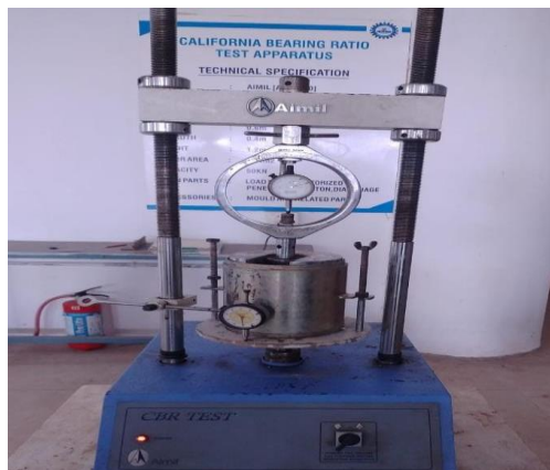
Figure 9 : CBR testing machine
