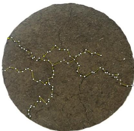
Fig. 8 Crack of soil + 20% fly ash
