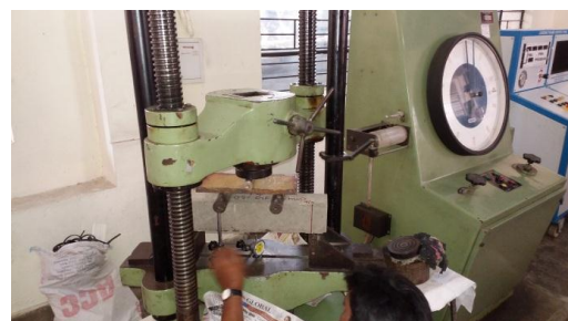
Fig. 4: Flexure Test Set Up
