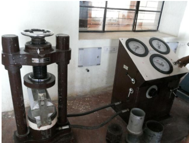
Fig. 2: Split tensile test set up
