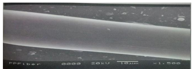
Fig.3. Scanning electron micrograph of polypropylene fiber
