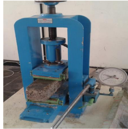
FIG.9: FLEXURAL TEST ON BEAM
