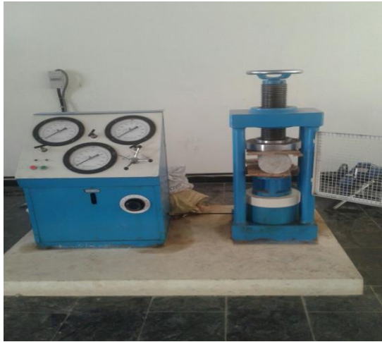
FIG. 6 :SPLIT TENSILE STRENGTH TEST ON CYLINDER
