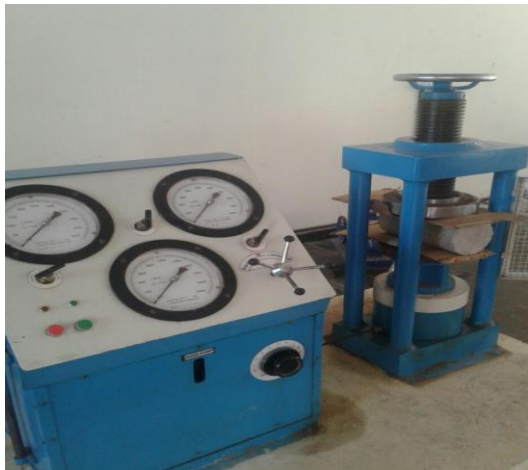
FIG 6:SPLIT TENSILE STRENGTH TEST ON CYLINDER
