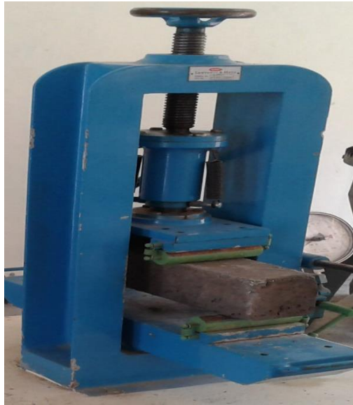
FIG.8:FLEXURAL TEST ON BEAM
