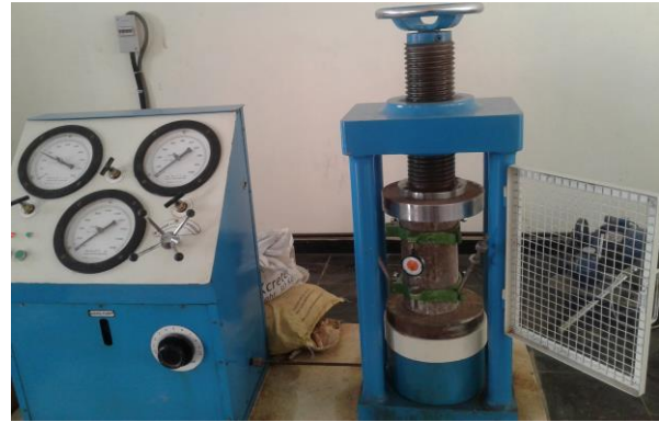
FIG.9: MODULUS OF ELASTICITY TEST ON BEAM
