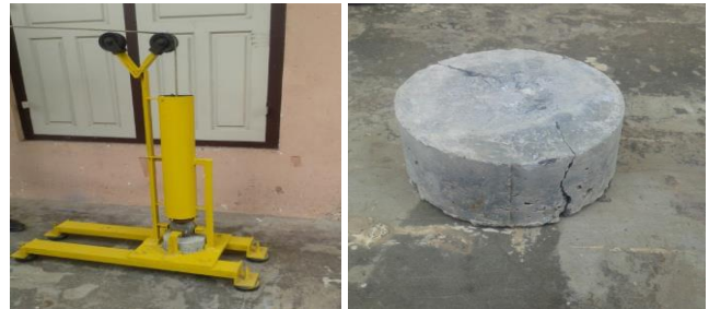
FIG.7:IMPACT RESISTANCE TEST ON DISC
