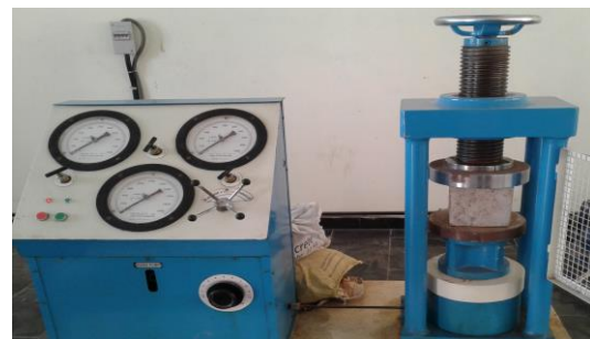
FIG.5: COMPRESSION TEST ON CUBE
