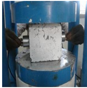
Fig.6 Ultrasonic Pulse Velocity Test Setup
