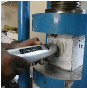
Fig.5 Rebound Hammer Test Setup
