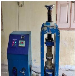
Fig.1 Compressive Strength Test Setup
