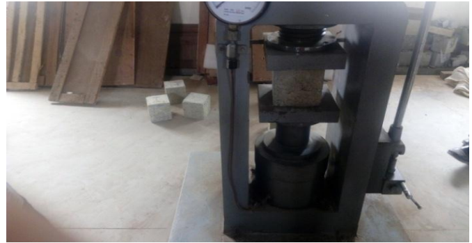
Fig. 2. Compression Testing of cubes
