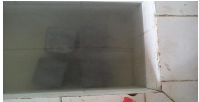
Fig. 3. Specimen subjected to water absorption
