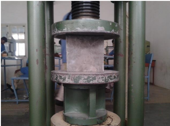
Figure 5.1: Compressive Strength test
