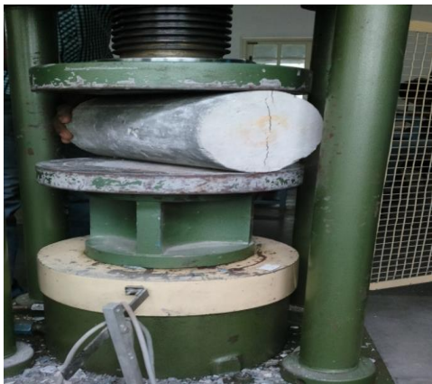
Figure .5.3: Split tensile Test
