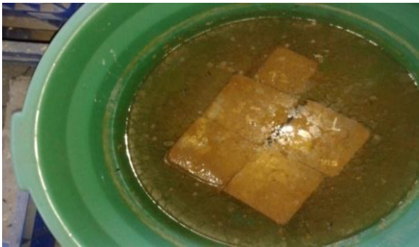
Fig.10. Specimens immersed in sulphuric acid solution
