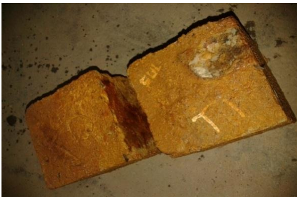
Fig.11. Formation of efflorescence
