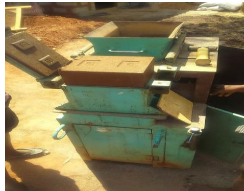
Preparing Mud Block
