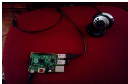
Fig 8. Raspberrypi wirelessly connected using WiFi dongle along with USB webcam
