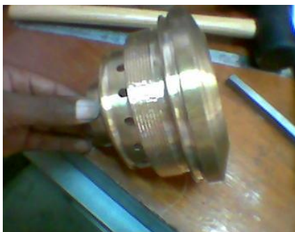
Fig. 10: Collimator assembly produced using the 3-Axis Supermax CNC VMC.
