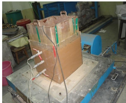
Figure 4. Soil Specimen in soil model with surcharge
