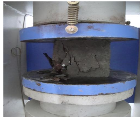
Fig. 1: Test Set up for Compressive Strength Test
