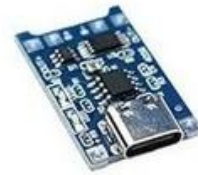
Fig -6: TP4056 Charging Module
