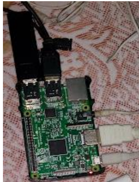
Fig. 1 Raspberry Pi 3B+ connected with power supply, display and different peripherals.
