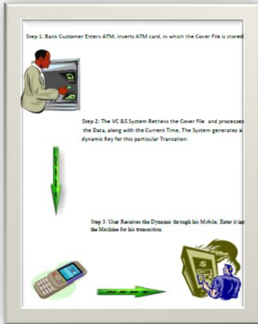
Fig 4.6: Authentication Process in a ATM Transaction.
