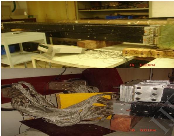
Figure.3. Practical Temperature rise setup
