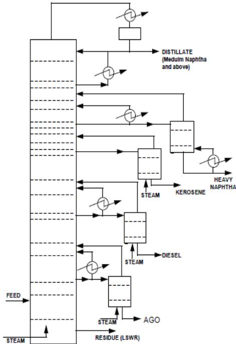
Fig.01 Schematic diagram of the crude oil distillation column.
