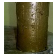
Fig.5. UCC soil sample in natural condition
