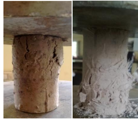
Fig.4 failure pattern before and after fibre reinforcement
