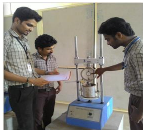
Fig 6: CBR Test Setup
