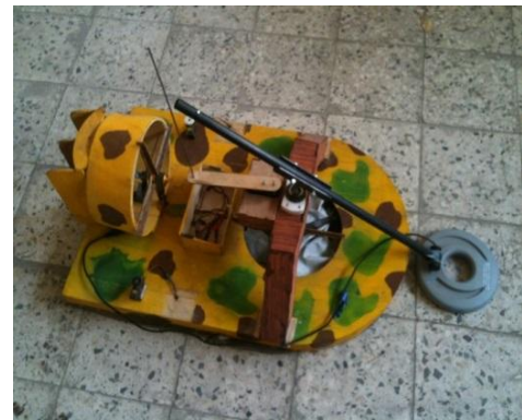
Fig (23) The hovercraft equipped with mine detector
