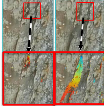
Figure 3. Visualization of rockfalls and the raveling detected by BlastVision® technology helps accurate analysis of slope response to the blast-induced vibration energy.
