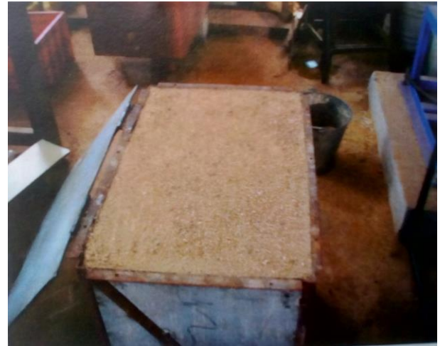
Fig 3.3 – Tank filled with sand for pullout test
