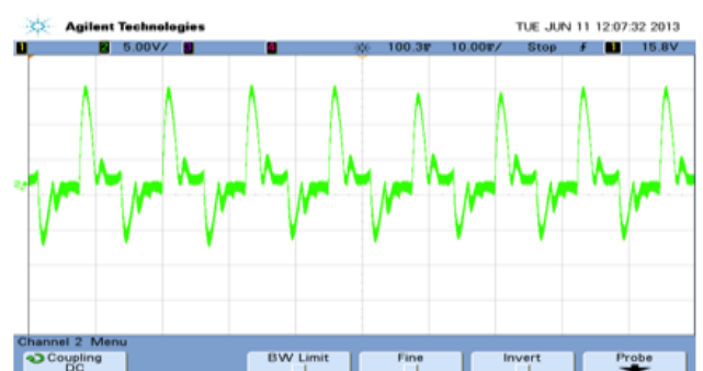
Fig 11: Stator current of R-phase
