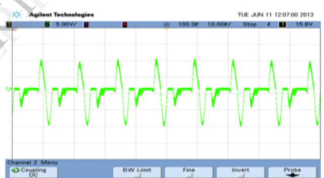
Fig 11: Stator current of R-phase
