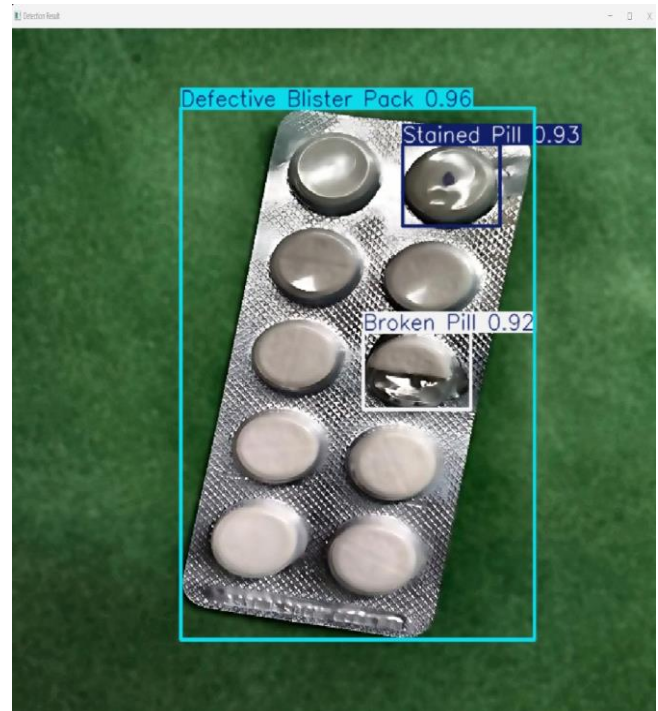
Fig. 9. Qualitative example of multi-defect detection within a single blister pack, showing simultaneous identification of defective blister pack, stained pill, and broken pill with corresponding confidence scores.
