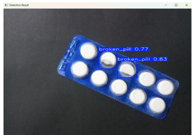
Fig. 7. Qualitative detection results under normal lighting conditions and tilted blister orientation.
