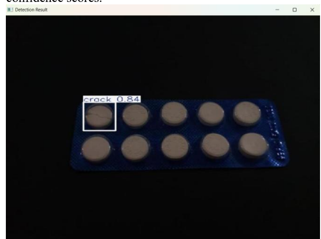
Fig. 8. Qualitative detection results under low-light conditions demonstrating robust defect detection.
