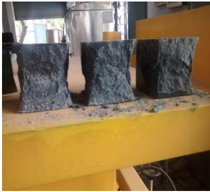
Figure 4: Failure of cube specimen without fibre
