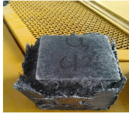
Figure 5: Failure of cube specimen with Steel with fibre
