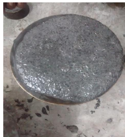
Figure 3: Flow of UHPGC mix
