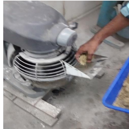
Figure 2: Addition of steel fibres
