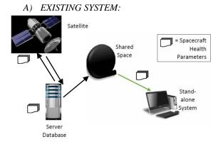
Satellites relay their overall health parameters to Spacecraft Checkout Server for Data Distribution Systems. These servers collect process and store the parameters in a shared space for access to all analysis packages. Any system accesses the shared space for the retrieval of parameters.<sup>[1]</sup>
