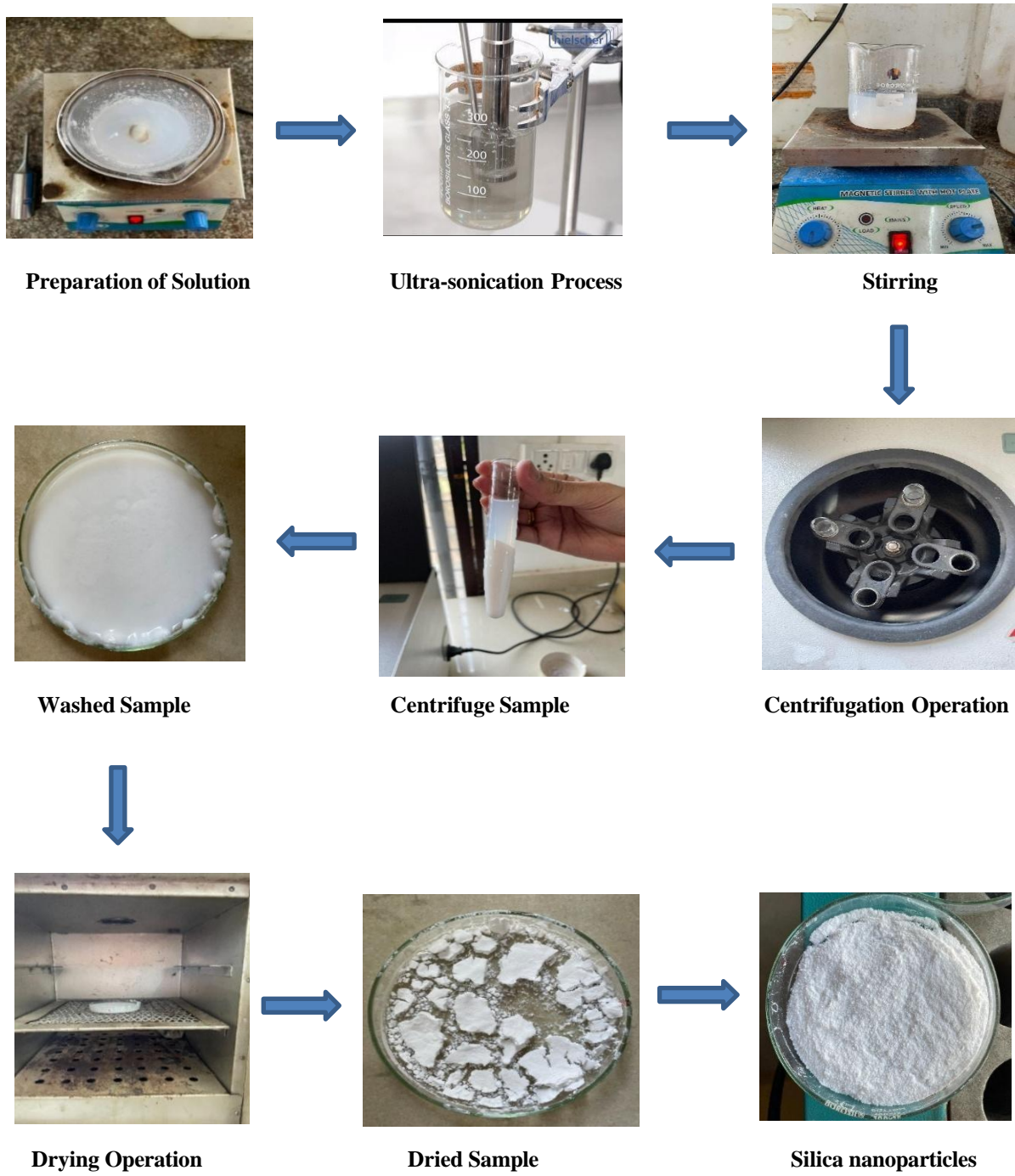
Figure No.1 Experimental Flow Diagram of Synthesis of Silica Nanoparticles
