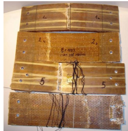
Fig. 16. Kinds of failure of full-scale SAS panels
