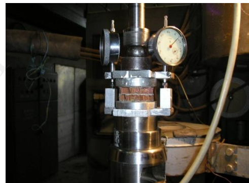
Fig.12. SAS samples during tests for compression along honeycomb height
