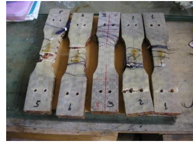
Fig.11. Typical failure at tension in SAS skin plane
