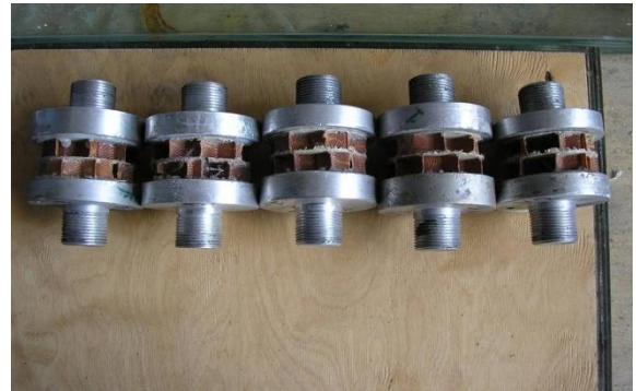
Fig.11. Typical failure at tension in SAS skin plane
