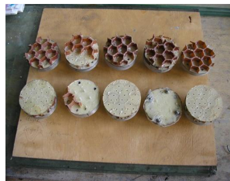
Fig. 13 Samples after testing for tension along honeycomb height
