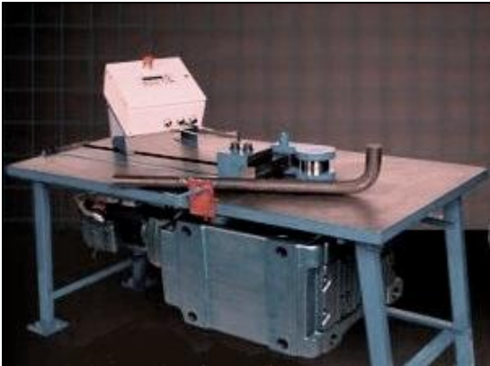
Figure 8. Machine jig for bending.
