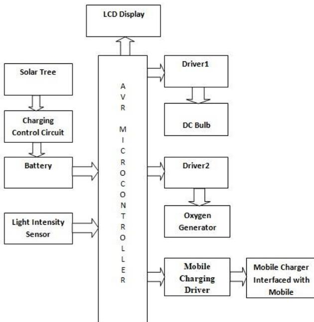
Figure 1: Block diagram of proposed method
