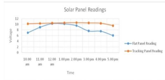
Figure 7. Graph of solar panel voltage with different time slots.
