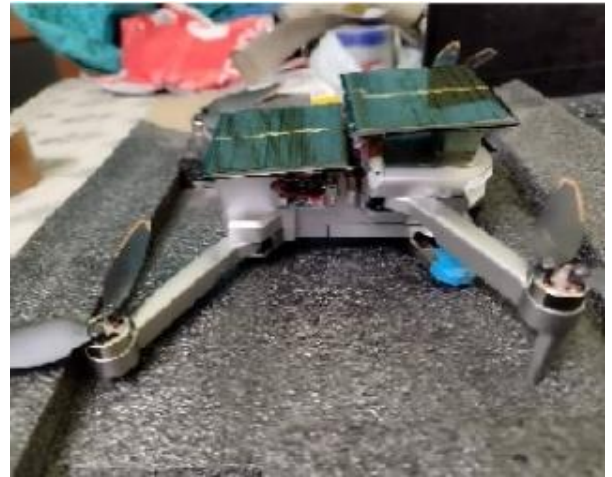
Fig. 10. Solar panels mounted for testing on a small commercial drone
