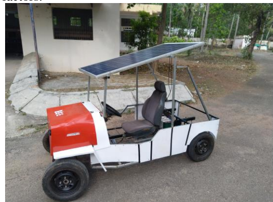
Fig 9 Prototype of Solar Powered Plug-In Electric Vehicle
