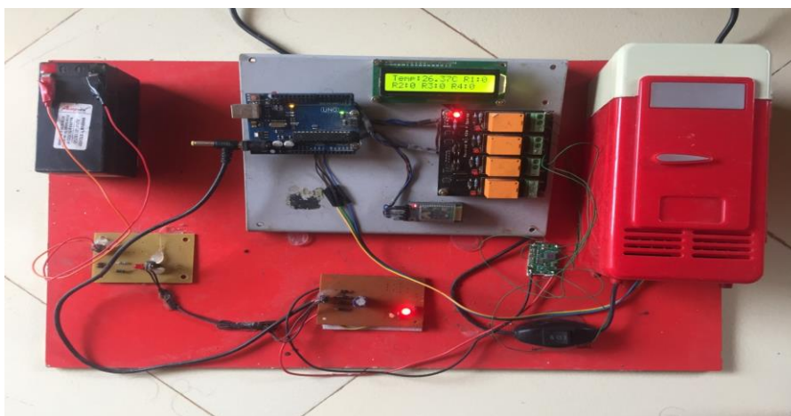
Working Fridge with temperature monitoring system
