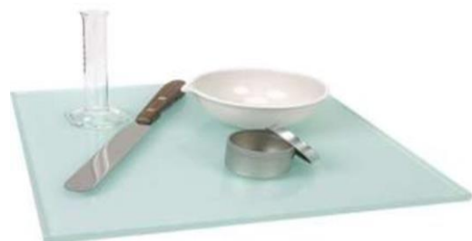
Fig.6.Plastic limit test setup
