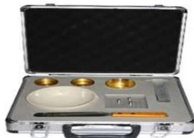
Fig.7.Shrinkage limit test setup
