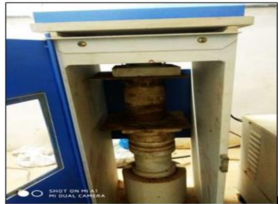
Figure 7: UCS Specimens are test in progress
