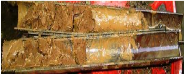
Figure.: Disturbed Soil Sample from SPT
