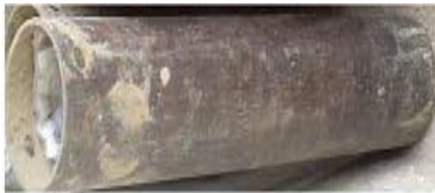
Figure.: Sample collected with casing
