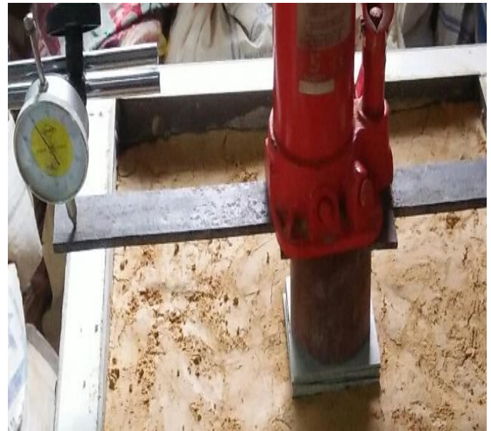
Fig 2 Setup for plate load test
