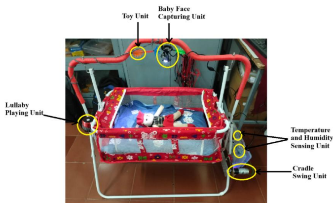
Figure 7. Photograph showing the actual physical implementation of various smart cradle units
