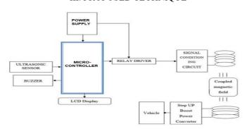
This paper proposes an enhanced resonant inductive coupling method to improve the efficiency of wireless EV charging by addressing key limitations such as energy losses, misalignment issues, and integration challenges with existing infrastructure. The proposed system leverages adaptive frequency tuning, optimized coil design, hybrid charging solutions, and smart grid integration to achieve higher power transfer efficiency and better adaptability across different operating conditions.
