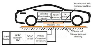
The architecture of a standard inductive wireless charging system for electric vehicles (EVs) adheres to the SAE J2954 standard, which outlines the framework for stationary wireless charging systems . This system comprises several key components that facilitate wireless power transfer.
