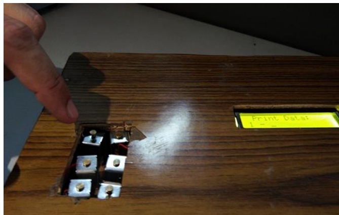
Fig. 6 Braille pattern generated on Solenoids
