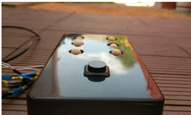
Fig.1 Braille Sensing Using Solenoid Actuators [1]
