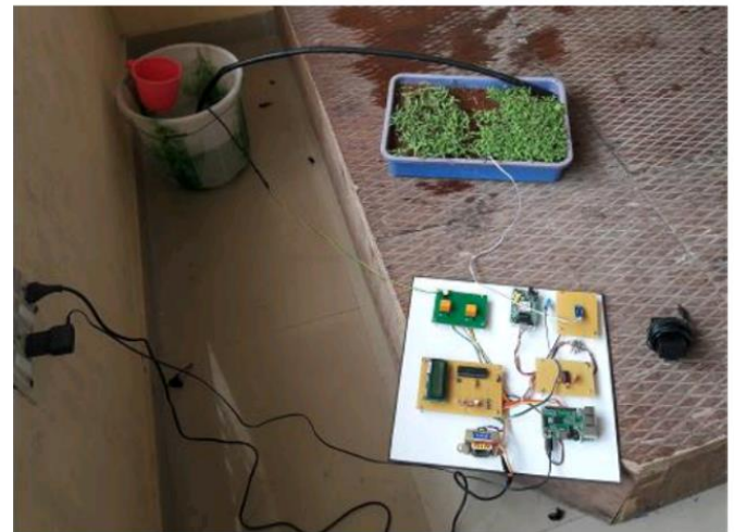
Fig.3. Smart Trickle Irrigation System
