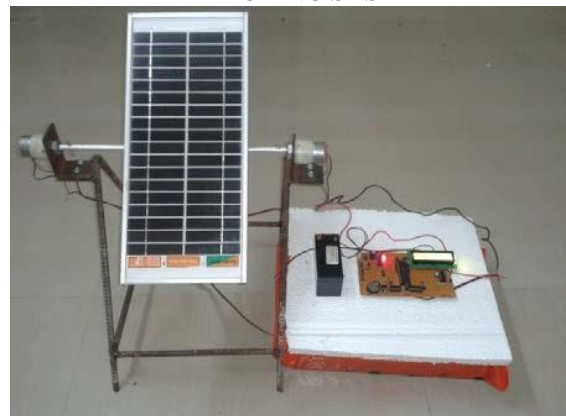
Fig.3 The prototype of time operated solar tracking system using RTC
