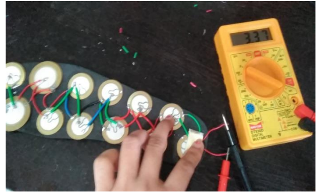
Fig. 4: Above figure shows the output of the piezoelectric sensor which is mounted on sole of shoes. In the proposed system twelve piezoelectric sensors are connected in parallel to generate electricity by foot pressure while walking. The sensor output can reach up to 4-5v and above as per users weight on foot. The different voltage readings take during this project as per the weight of the user are shown in table 1.
